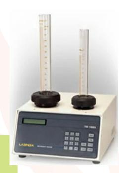
Tap density tester is designed to measure the tapped volume and/or density of powders, granules and other similar products.
